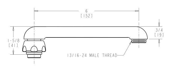
DIMENSIONS ARE IN INCHES AND [MILLIMETERS].
