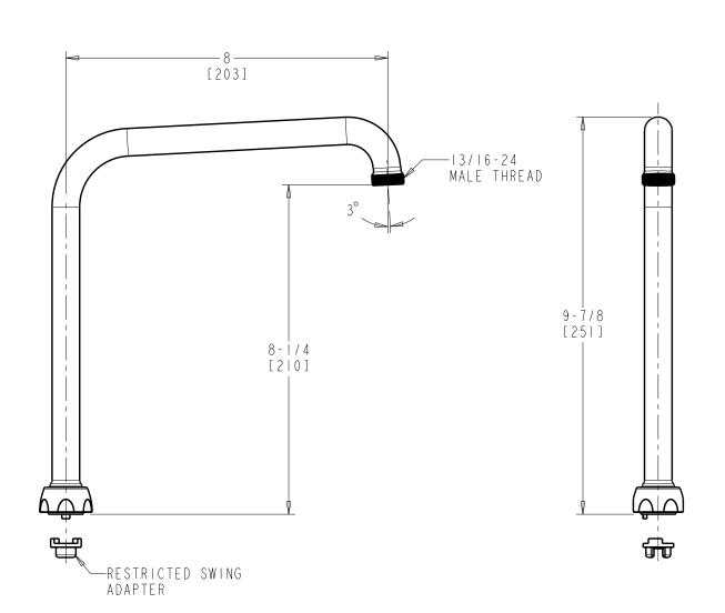
DIMENSIONS ARE IN INCHES AND [MILLIMETERS].
