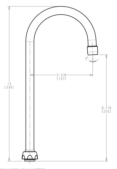
DIMENSIONS ARE IN INCHES AND [MILLIMETERS].
