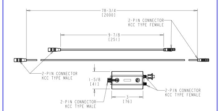
DIMENSIONS ARE IN INCHES AND [MILLIMETERS].
