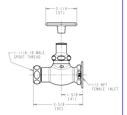
DIMENSIONS ARE IN INCHES AND [MILLIMETERS].
