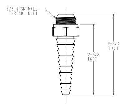
DIMENSIONS ARE IN INCHES AND [MILLIMETERS].
