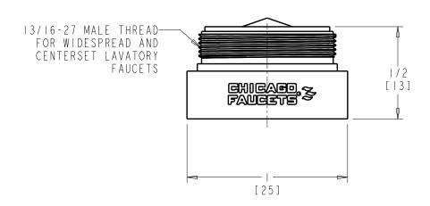
DIMENSIONS ARE IN INCHES AND [MILLIMETERS].
