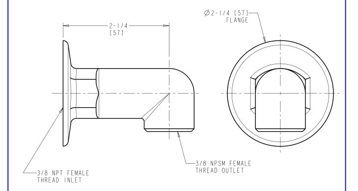
DIMENSIONS ARE IN INCHES AND [MILLIMETERS].
