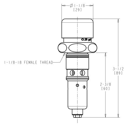
DIMENSIONS ARE IN INCHES AND [MILLIMETERS].
