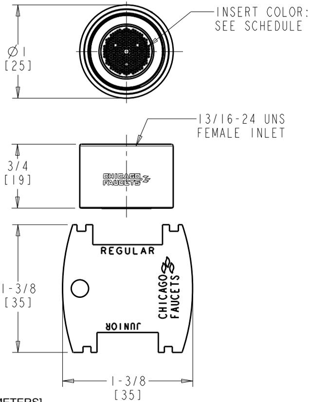
DIMENSIONS ARE IN INCHES AND [MILLIMETERS].
