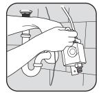
1. Connect SSPS unit. Attach to faucet and install water supply line.
