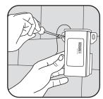
4. Insert anchors into holes and mount LTPS unit to wall with supplied screws.
