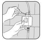
5. Secure SSPS to wall. Insert anchors into holes and mount SSPS unit to wall with supplied screws.
