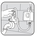
Attach inlet hose to supply and turn on water. With water on, check system for leaks.\*
