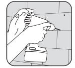
Drill holes for screw anchors.
