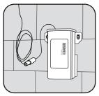
Connect spout wire to LTPS connector wire, making sure connectors are oriented correctly.
