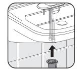
3. Mount bracket from underneath. Place hoses through large opening and mounting rod through small opening. Make sure flange sits securely against surface.
