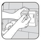
2. Position LTPS unit on wall and mark mounting holes on mounting surface.
