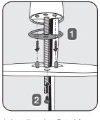
1. Install gasket flat side down. If installing a cover plate, align holes in spout base with pins on plate. Feed the power cable and braided hose through plate. Secure plate to spout.
