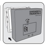
3. Reinstall the control box cover and secure it with the #2 Phillips screw.
