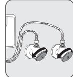
3. Open supply stops and check for leaks. Water may run through spout.
