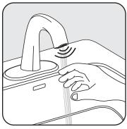
1. Once wiring is complete, the red 2. Adjusting the Water Temperature b. Cap must be partially pulled from sensor light at the outlet will glow for 5 seconds. After the light switches off, place your hands in front of the faucet to activate.
