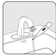
D. Mixed water temperature must be checked at the point of use and the mixing valve adjusted to ensure delivery of water at a safe temperature not exceeding 110°F (43°C). Water temperatures in excess 110°F (43°C) are dangerous and may cause scalding, severe injury or death!
