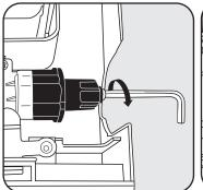
a. Loosen the cap screw until the handle turns freely (do not remove the screw) with a 3mm (7/64") hex
