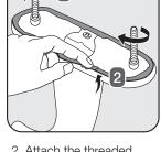
2. Attach the threaded rods to bottom of the cover plate. Apply sealant to underside of the cover plate where shown.
