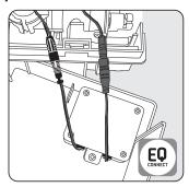
2. Connect wiring connectors, gray to gray, black to black. Snap into the wiring harness Tuck the completed green connection into the space as shown.
