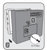
cover by using a #2 Phillips screwdriver to loosen the cover screw.
