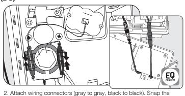
completed connections into wiring harness.
