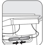
ii. Connect blue connector on SSPS to blue connector on the turbine and tuck them into the cavity as shown.
