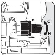
the valve to adjust temperature. Turn the handle clockwise to decrease temperature or counter-clockwise to increase temperature.
