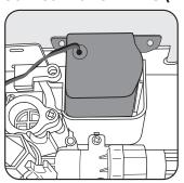
1. Insert LTPS into control box upper compartment, aligning slots with compartment ribs. Attach wiring connectors green to green, gray to gray.
