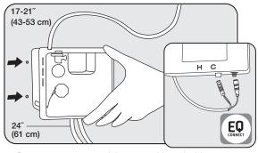
1. Determine position of the control box, hold it against the wall and mark the locations of the two mounting
