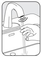
1. Once wiring is complete, the red sensor light at the outlet will glow for 5 seconds. After the light b. switches off, place your hands in front of the faucet to activate.
