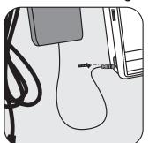
1. Choose a location and mount the transformer. Run the cable from the transformer through opening in control
