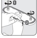
2. Attach the threaded rods to bottom of the cover plate. Apply sealant to underside of the cover plate where shown.
