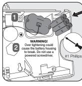
1. Open battery housing and insert batteries according to diagram inside housing. Replace battery cover. Do NOT overtighten screws.
