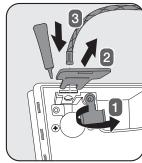
1. Remove the control box 2. Pivot yellow locking tab and remove metal key at top of box. Apply silicone-based lubricant to the end of the spout hose and insert it through the hole.
