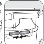
i. Insert SSPS power supply into control box upper compartment. Attach connectors, gray to gray, black to black. Snap the completed connections, into the wiring harness as shown.
