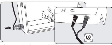
1. Bring wire into box. Snap wire into holder on side of box.
