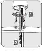
1. Install gasket flat side down. If installing a cover plate, align holes in spout base with pins on plate. Feed the power cable and braided hose through plate. Secure plate to spout.
