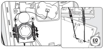
2. Attach wiring connectors (gray to gray, black to black). Snap the completed connections into wiring harness.
