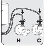
2. Attach 3/8" compression supply hoses from control box to the supply stops. Wrench tighten.
