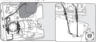
1. Insert LTPS into control box upper compartment, aligning slots with compartment ribs. Attach wiring connectors green to green, gray to gray.
