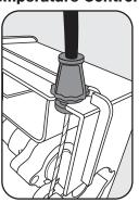
2. Slide black riveted attachment into the groove of the control box and push back into large opening.
