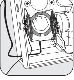
2. Attach wiring connectors (gray to gray, black to black). Snap the completed connections into the wiring harness as shown.
