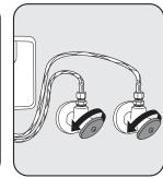
3. Open supply stops and check for leaks. Water may run through spout.
