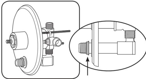
3. Position 2-hole round trim over valve and pipe and attach with screws. Insert pipe and drain seal with larger diameter end closest to the trim.
