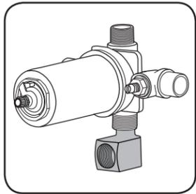
1. Install valve with brazed elbow.
