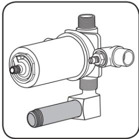
2. Install straight nipple 1/2" pipe – 1/2-14 NPT both ends. Use pipe sealer on both ends of pipe nipple. Tighten securely with wrench. Take care not to damage chrome plate finish.
