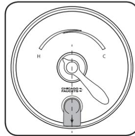
4. Make sure drain holes are lined up vertically and drain cap is tightly secure.
