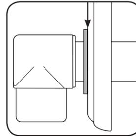
5. Push seal inside the drain back opening until it seats flush against the drain body.
