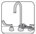
2. Place spout onto valve body until fully seated. Tighten spout nut with wrench. Connect water supplies, flush line, and attach outlet.
