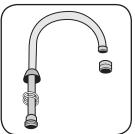
Remove outlet from spout. Place two split rings on spout near the base. Slide spout nut onto spout.
