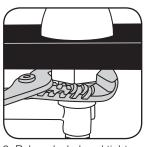
9. Below deck, hand tighten the flanged nuts and then with a wrench tighten 1/4 - 1/2 turn more.
