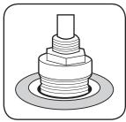
6. Above deck, place a sealing washer over each handle stem and around the cartridge housing.
