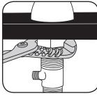
8. Below deck, hand tighten the flanged nuts and then with a wrench tighten 1/4 - 1/2 turn more.
