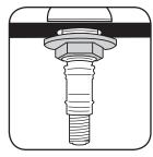
3. From below deck, use nut and metal washer to secure spout to deck. Hand tighten.
