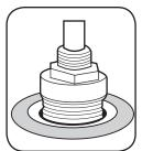
5. Above deck, place a sealing washer over each handle stem and around the cartridge housing.
