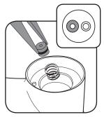
4. Remove hot orifice seat using needle nose pliers. The hot orifice seat is on the left.
