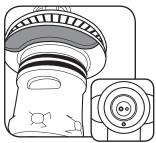
5. Align mounting pin to groove in brass nut when replacing cartridge assembly. Pin orientation should face front.
