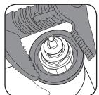
2. Loosen cartridge assembly using channel
