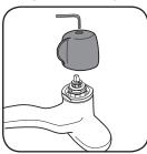
1. Using wrench, remove hex screw and handle. Depress actuator stem to purge any residual pressure.
