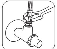
6 Install Outlet - Using outlet key, turn outlet clockwise until tight.
