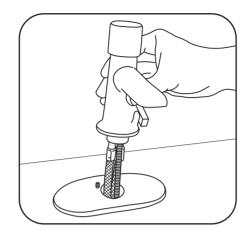
Feed supply hoses through faucet mounting bracket. Slide bracket over faucet mounting bolt and secure to sink.
