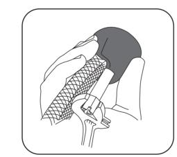
Flush lines at supply stops and attach to outlet. Insert filters into ends of each supply line. The blue sticker indicates the cold water supply hose.
