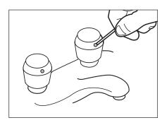
**Step 9** Replace handle, tighten handle nut with allen wrench and replace index button.
