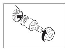
**Step 1** Push each cartridge into valve body until it seats. Add cap nuts and hand tighten. Add handles.
