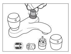
**Step 6** Place new filter, screen and MVP cartridge in valve body.
