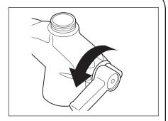
**Step 2** Rotate RIGHT handle (and cartridge) counter clockwise to the desired closed position.
