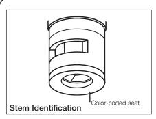
Ensure cartridges are in the closed position before installing into valve body.
