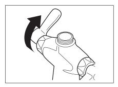
**Step 4** Move LEFT handle (without moving cartridge) to the open position and fully tighten right cap nut to 20 to 27 ft. lb. torque. Return handle to closed position.
