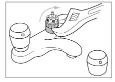
$\textbf{Step 7 and 8} \ \ \text{Replace cap sealing washer and actuator assembly.} \ \ (\text{Adjust flow cycle as described in } \#3.) \ \ \ \text{Do not over tighten cap.}$
