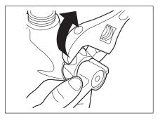
**Step 3** Using handle to maintain stem position, fully tighten right cap nut to 20 to 27 ft. lb. torque.
