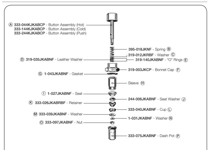
No. 333-X NAIAD is used for all No. 333 Basin faucets and all push button stops and contains a fast closing dashpot. Note: 333-XSLO is the same as No. 333-X, but with an additional external timing feature located on the button and a 333-073KJKNF adjustable slow closing dashpot.
