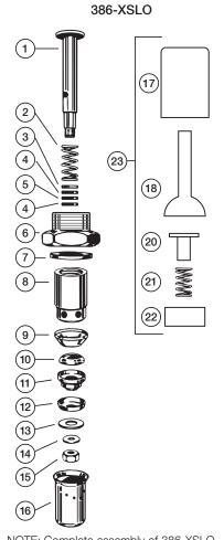
NOTE: Complete assembly of 386-XSLO cartridge and 386-010K Oscillating Lever Handle assembly for Urinal Valves.
