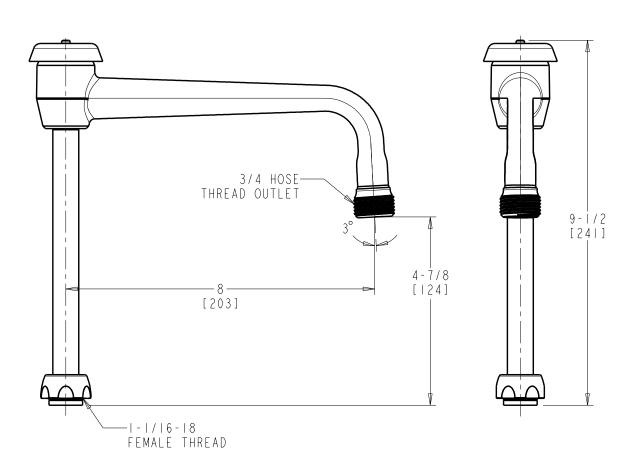
DIMENSIONS ARE IN INCHES AND [MILLIMETERS].
