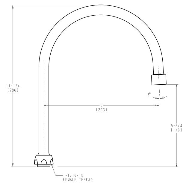
DIMENSIONS ARE IN INCHES AND [MILLIMETERS].
