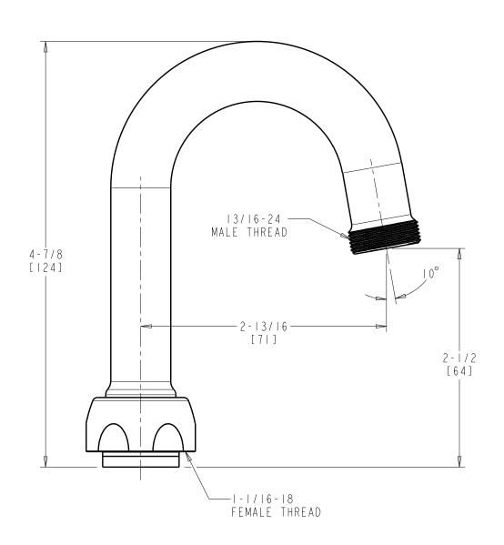
DIMENSIONS ARE IN INCHES AND [MILLIMETERS].
