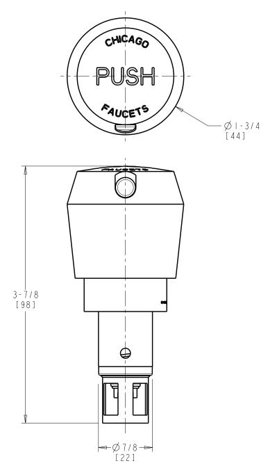
DIMENSIONS ARE IN INCHES AND [MILLIMETERS].
