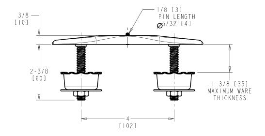
DIMENSIONS ARE IN INCHES AND [MILLIMETERS].
