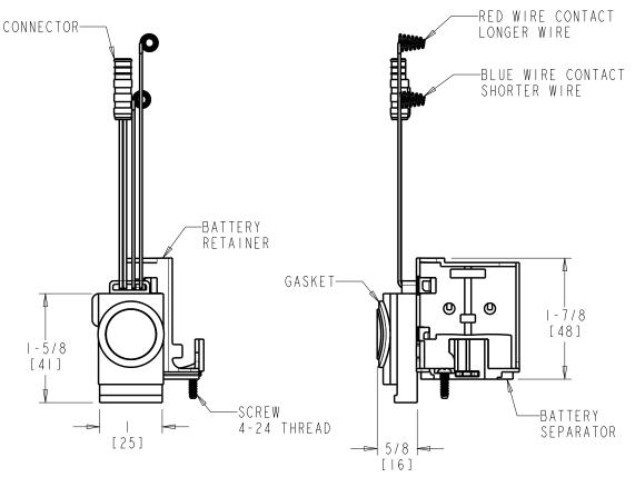
DIMENSIONS ARE IN INCHES AND [MILLIMETERS].
