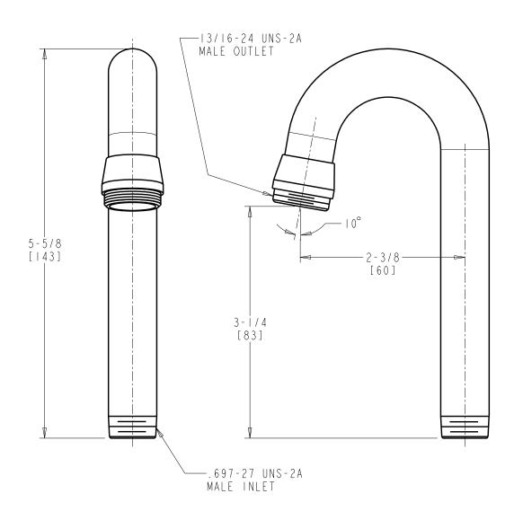
DIMENSIONS ARE IN INCHES AND [MILLIMETERS].
