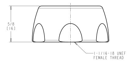
DIMENSIONS ARE IN INCHES AND [MILLIMETERS].
