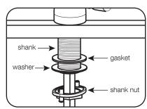
4. Below the sink, slide gasket and washer over shank. Hand tighten shank nut to hold faucet in place. Check faucet position. Secure nut with screwdriver by tightening screws on both sides of nut. Note: You may also tighten the shank nut with a basin wrench. DO NOT overtighten.
