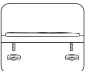
Below sink, secure cover plate with black mounting bolts on each post.
