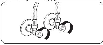
Flush lines and attach the compression hoses to the supply stops with wrench. Do not overtighten. Hoses are color coded, red for hot and blue for cold.
