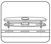
Install two posts into bottom of cover plate. Position cover plate and gasket over holes in the sink.
