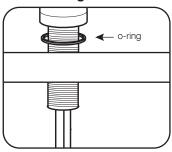
Position large o-ring in groove at bottom of spout. Insert faucet hoses and shank through sink hole.
