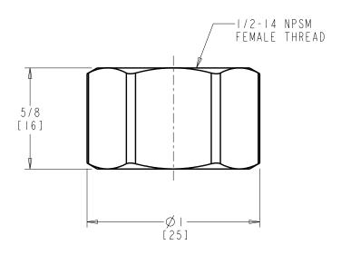
DIMENSIONS ARE IN INCHES AND [MILLIMETERS].
