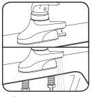
4. Remove outlet and flush lines.
